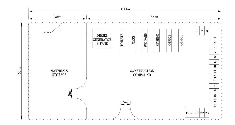
PLAN VIEW OF INDICATIVE CONSTRUCTION COMPOUND ARRANGEMENT
